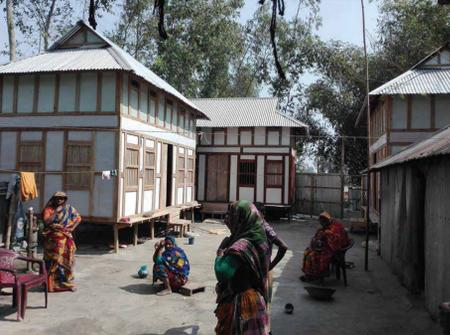
Adopting a co-design, test and demonstrate approach, the climate and flood resilient housing concept was piloted. 12 houses were retrofitted on raised plinths with facilities for sanitation, clean drinking water, and homestead garden.
